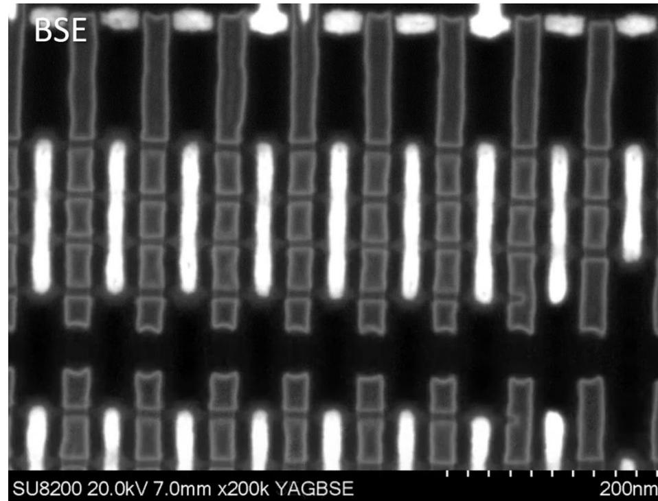
14-nm FinFET SRAM under electron microscope
